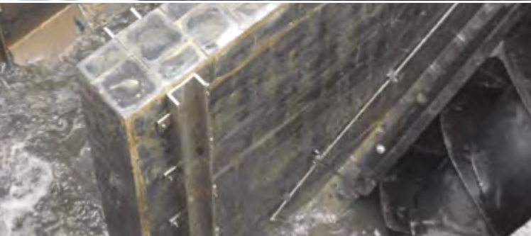
Floor and side wall linings with cast basalt (pictured left) or with hard ceramic (pictured above).
