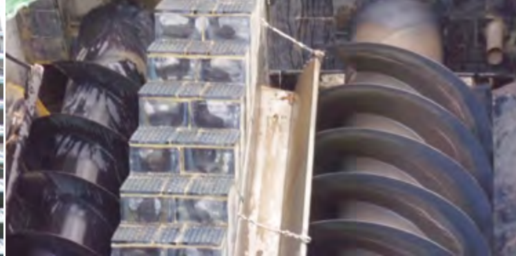
Spiral trough with cast basalt lining
